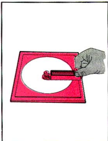
Cutting circular gasket compass-style.
